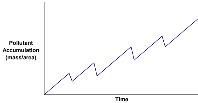
Figure 4.26 Unchecked pollutant accumulation arising from an inappropriate set of buildup and washoff parameters
